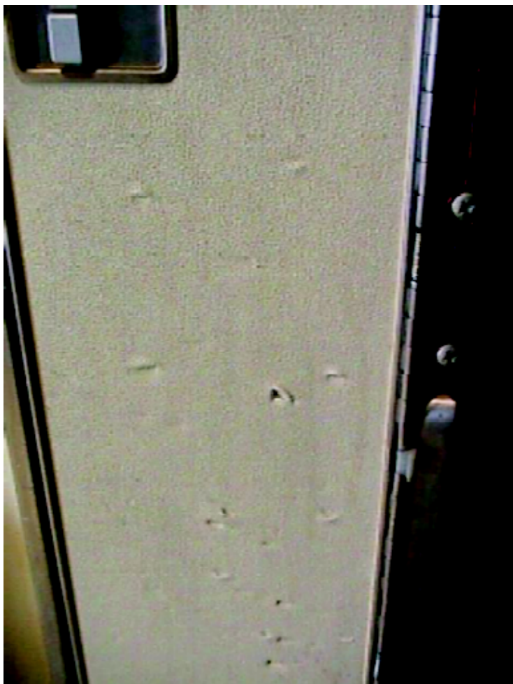
Extensive Damage on Tedlar Figure 6010/GRAPHIC 25-23-37-300-010-A01
